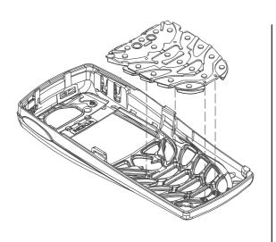
Remove Keypad (only if it is necessary to replace keypad).
