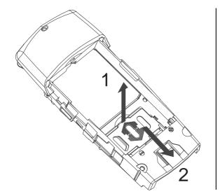
Remove SIM cover (only if it is necessary to replace SIM cover).
